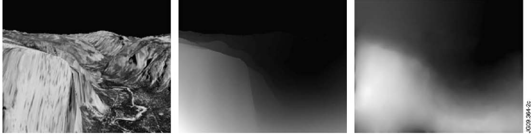
Fig. 2. Yosemite sequence [23]: image 7 in the sequence (left), modulus of the velocities used to generate the transition from image 6 to image 7 (middle) and modulus of the reconstructed velocity field obtained by applying the optical flow method to the image pair image 6 to image 7 (right).
